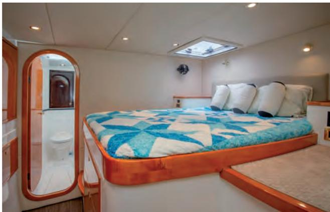
*The forward cabins are set athwartships, enabling the hulls to be kept nice and narrow.*
